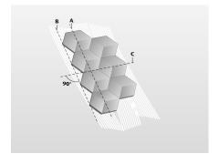
To be able to regulate the laying direction of the starting rows, the edges of the tiles must be in line with the working line B.
